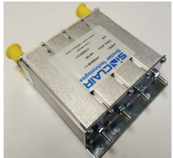
Figure 14, Illustration comparing a bandpass filter curve with a preselector filter curve on the left, Photo of a typical preselector made up of four cavity filter sections is on the right
