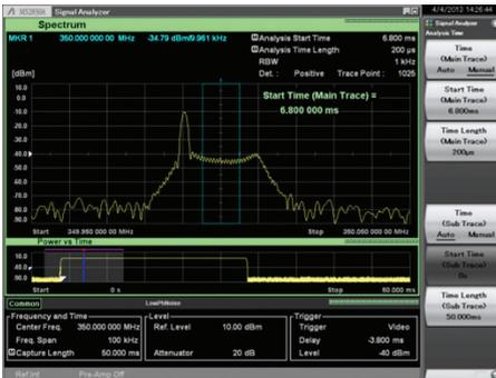
Figure 66: 2-FSK signal instantaneous Spectrum-3
