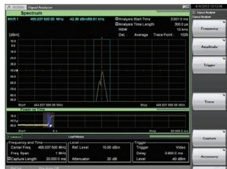
Figure 57: Spectrum transition immediately after Start-2
