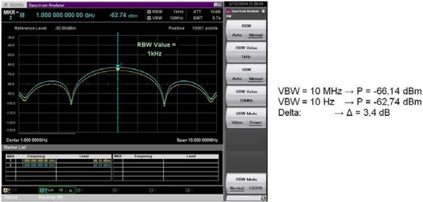
Figure 94: Signal under test measured with RBW 1000 kHz / VBW 10 MHz and 10 Hz and an average factor of 10
