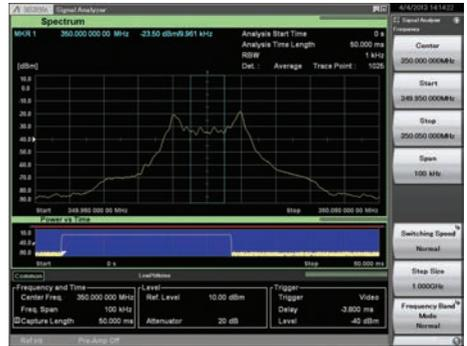
Figure 68: 2-FSK signal spectrum (Signal analyzer)
