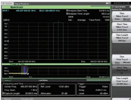
Figure 56: Spectrum transition immediately after Start-1
