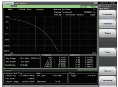
Figure 17: Example of CCDF trace (CCDF of terrestrial digital TV signal)
