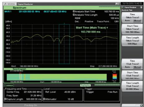
Figure 75: Instantaneous spectrum at power-on
