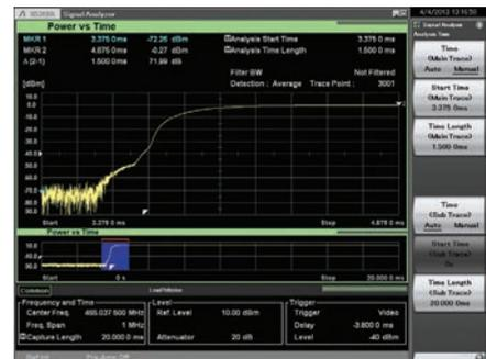
Figure 60: Change in power with time (Signal Analyzer)
