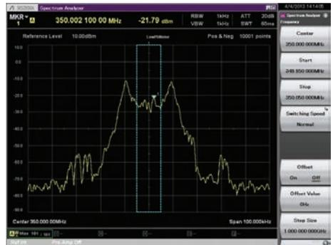
Figure 69 : 2-FSK signal spectrum (Spectrum analyzer)
