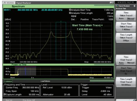
Figure 67: 2-FSK signal instantaneous Spectrum-4
