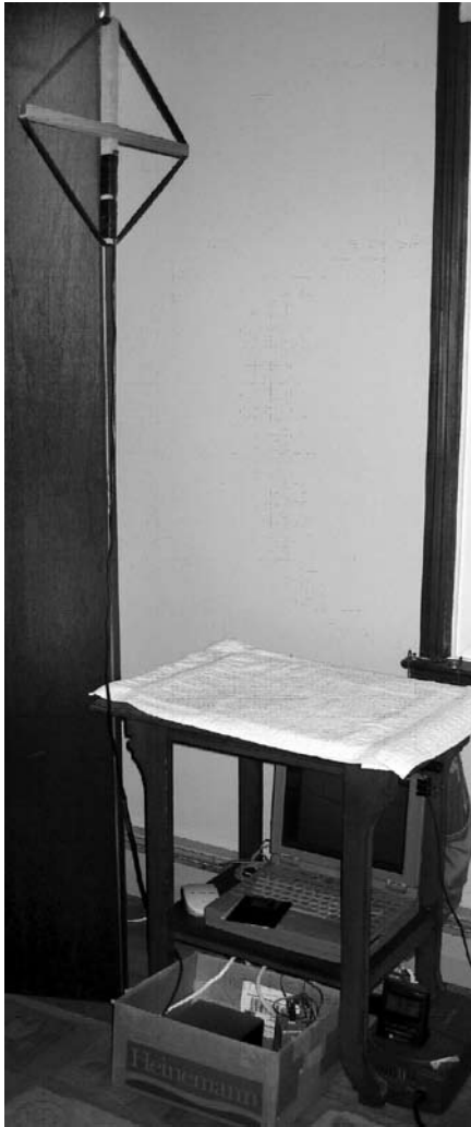
Figure 7 — This photo shows my complete system, with the loop antenna at top left, a computer on a shelf and the VLF radio and analog to digital converter device in a box below the computer.
