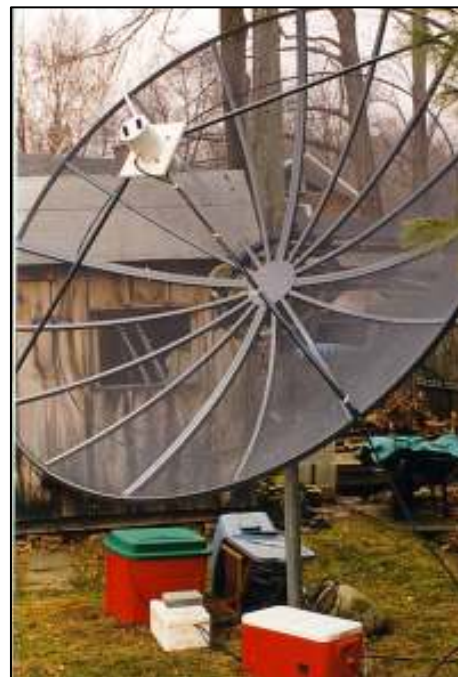
My 1420 MHz Total Power Telescope – 10' dish with horn leading to temperature controlled LNA, IF Amp, detector (in cooler), then leading to voltage amp (foam box), then to A/D device and computer (in plastic bin). Power supplies are on wooden stand.
